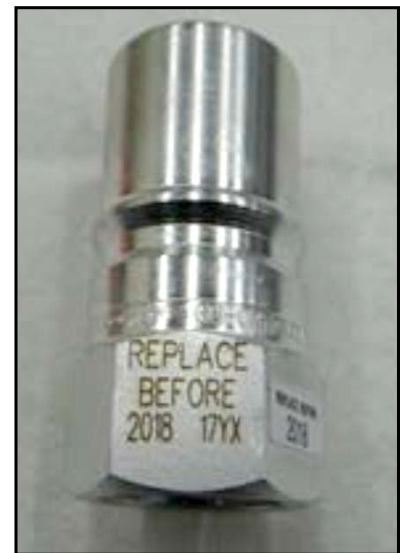
Replacement date marking and decal on male segment of the Pioneer coupler.
