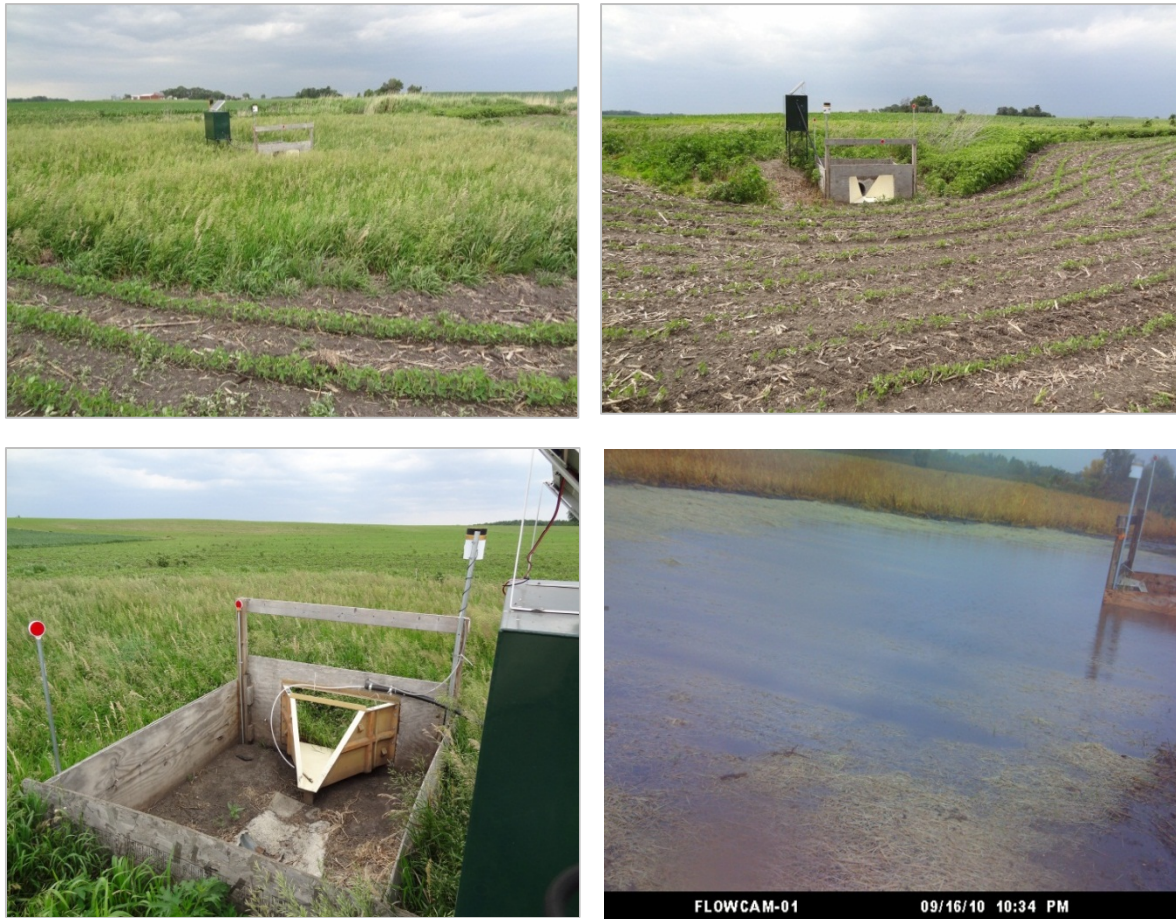
Figure 17. (Top Left) Surface water monitoring station located behind a 30-foot grass filter strip. (Top Right) Surface water monitoring station on control watershed with no filter strip. (Bottom Left) Surface water monitoring station with flume for runoff rate measurement and instrument cabinet containing sampling equipment. (Bottom Right) Pondered water in front of flume following a larger rainfall event in September 2010.
