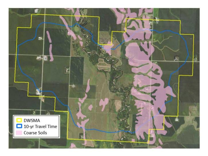
This map shows the boundary of the Rock County Rural Water DWSMA. The yellow line marks the DWSMA boundary. Within this area, adoption of the BMPs listed on pages 2-3 is needed. The pink areas are coarse soils. Where the coarse soils are the dominant soil type within a field, the BMPs for coarse soils should be followed. Areas that are not identified as having coarse soils should follow the fine textured soil BMPs.
