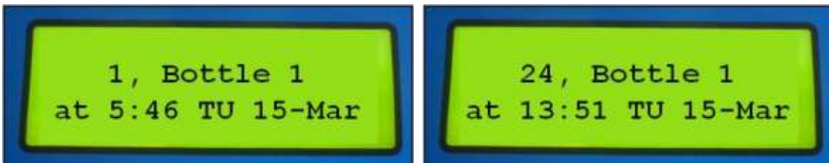
Figure 9. Pulse #, Bottle #, and sample date and time readout of the ISCO 6712 Automatic Sampler. The two images above represent the start and stop times for bottle #1.
