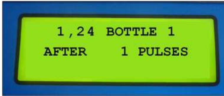
Figure 10. Autosampler default display screen for a resumed/restarted program. This shows that when triggered again from the datalogger, the sampler will begin with 1 of 24 pulses on bottle #1.
