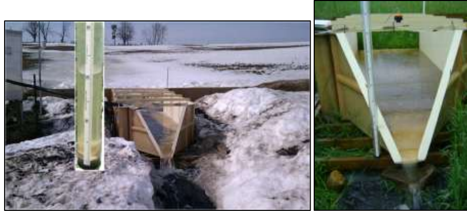
Figure 4. Transparency tube photos during runoff.
